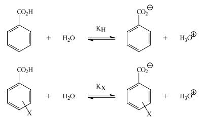
The Hammett Equation relates the relative magnitude of the equilibrium constants to a *reaction* constant  $\rho$  and a substituent constant  $\sigma$ .
