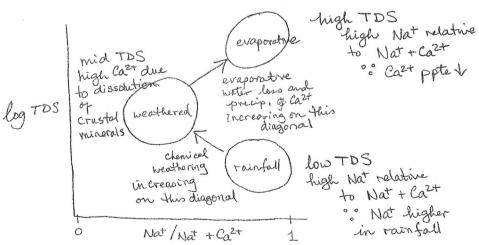
**Solution:** Using a spreadsheet and the data given in the question to calculate the TDS and the  $Na^+/(Na^+ + Ca^{2+})$  ratio for each of the four major river systems.
