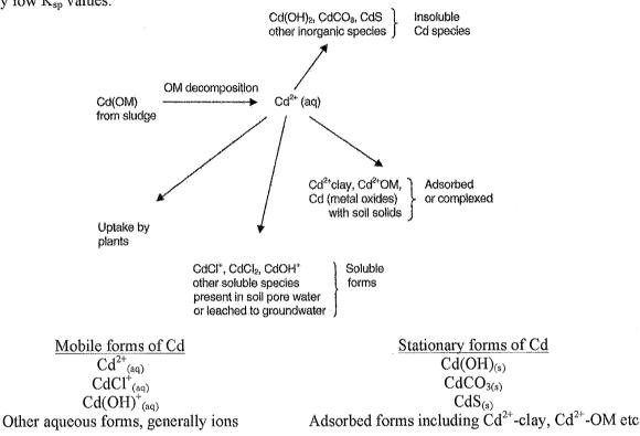
Note: Most of the stationary forms of insoluble d species, become more water soluble in acidic solution. This is because the anions produced upon dissolution (e.g. OH,  $CO_3^{2-}$  and  $S^{2-}$ ) are basic and therefore reaction with  $H^+$ .
