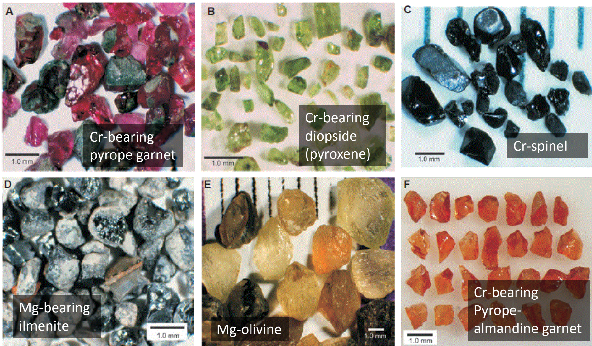
FIGURE 5. Examples of typical colours and surface features of kimberlite indicator minerals: (A) purple and mauve Cr-pyrope, some retaining kelyphite (dark); (B) emerald green Cr-diopside; (C) opaque black Cr-spinel, some exhibiting slightly resorbed octahedral form; (D) black Mg-ilmenite, both single crystals and polycrystalline morphologies shown; (E) yellow Mg-olivine; (F) orange eclogitic pyrope-almandine garnets. Photos A to E from the Geological Survey of Canada, photo F from Mineral Services Canada.
