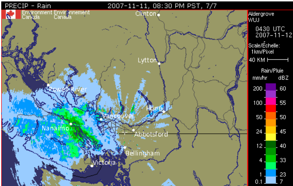
Radar rainfall rate estimates for southwestern British Columbia at 8:30 PM on Nov. 11, 2007. The highest rates are in the Nanaimo area, and are between 4 and 12 mm/hr. The radar instrument for this map is located near Abbotsford.
