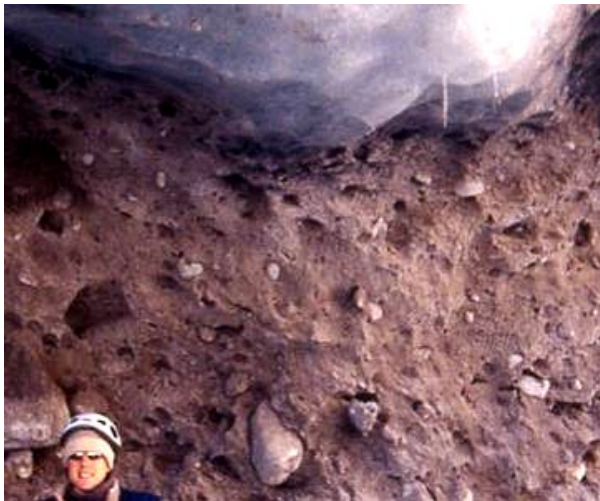
Glacial till at the front of a glacier in Iceland. Note absence of layering and sorting, and angular shape of many of the clasts. This material is rich in clay and is quite strong.
